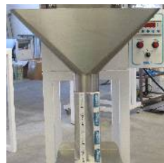
Additional discharge chute
