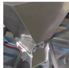
Discharge chute + timing hopper
