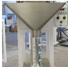
Additional discharge chute
