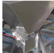
Discharge chute + timing hopper
