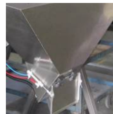
Discharge chute + timing hopper
