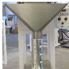
Additional discharge chute
